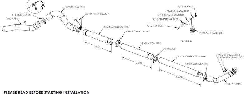
MBRP Inc. has made every effort to ensure that all components of this system are of superior quality and properly packaged. It is the installer's responsibility to ensure that all components are present and fit together as shown. Please also ensure that all components are undamaged before removal of the factory exhaust. Finally, check that this system properly matches the make and model of the vehicle and will not interfere with previous or planned modifications.
